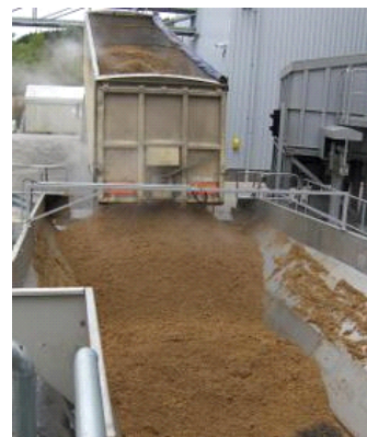
The plant utilises draff, which is a by-product from whisky production. This comes from 17 different distilleries and is mixed 50/50 with wood chips.
