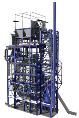
A 3D illustration of the Boehringer Ingelheim plant, with the boiler at the bottom and the filter at the top.
