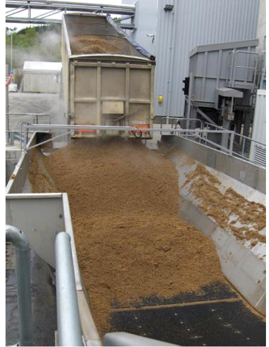
The Helius CoRDe Rabobank CHP plant processes and burns solid residues from the malt whisky distilling process, known as draff, together with clean wood. Annual fuel input is approximately 115,000 tons of wet draff from local distilleries and 60,000 tons of uncontaminated wood chips. Power is exported to the grid and heat is utilised for draff fuel drying as well as in the whisky process.
