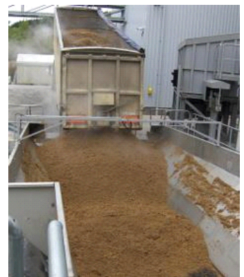
The plant utilises draff which is a by-product of whisky production. This comes from 17 different distilleries and is mixed 50/50 with wood chips.
