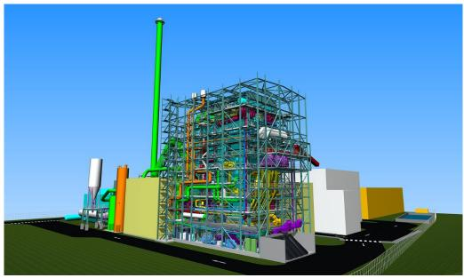
A 3D illustration of the highly efficient AET combustion system at Tilbury Green Power.
